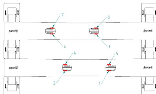
Now start to finish the welding on each side of the stubs, see blue marking.
